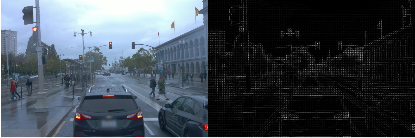
Figure 7. Visualization of HOG Feature Descriptors. The lines in the right image show the gradient directions with the highest magnitudes of each histogram.
